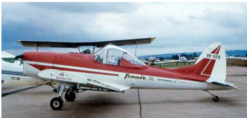
In 1965 Chippy was converted as third SA-29 Spraymaster at Bankstown, Australia, and recertificated as VH-GEB. Mods include forward part of fuselage interior and front seat removed to install a hopper, rear seat raised, and single seat bubble canopy installed. It also received a dorsal fin, Scott-style tailwheel, and attachments for spray equipment and controls (skin holes and doublers still very much in evidence today!) It still had the stock 145-hp Gipsy Major engine. It flew out of Tintinara, Southern Australia, landed in a field and was badly damaged. Once repaired, it continued to operate as a Spraymaster until 1969.
