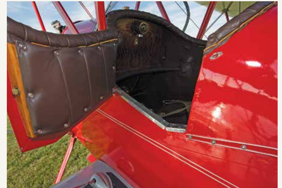
Entrance to the front pit is made easier by a small door.
