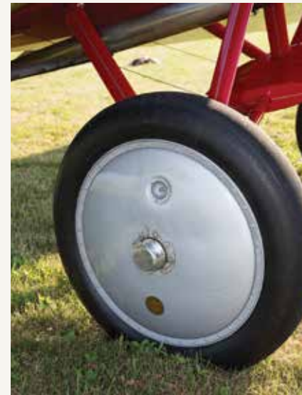
30 x 4 tires are correct, but, while crop dusting, many Travel Airs ran on truck tires.
