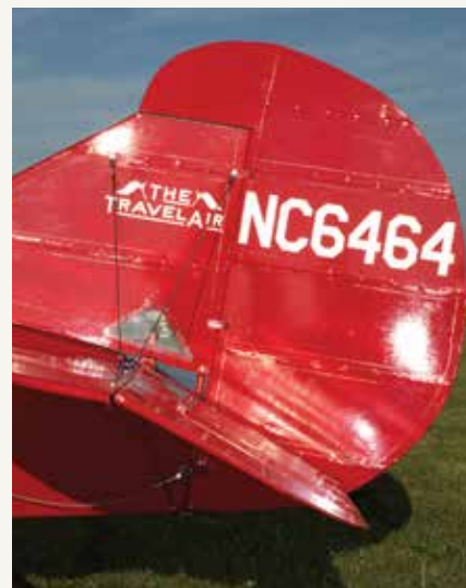
The massive tail gives excellent control down to almost zero airspeed.
