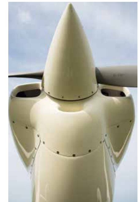
The nose bowl, a Meredith design, is for max cooling and looks.
