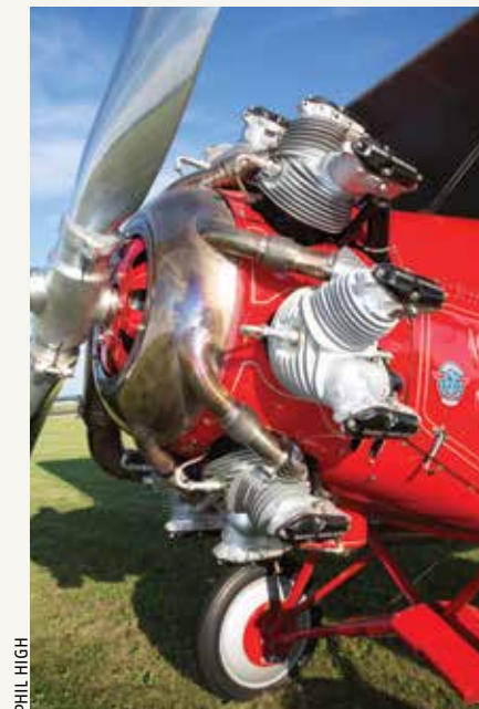
The Wright R-760 is a later version of the original J-6.
